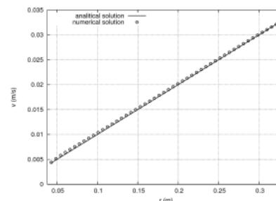
A comparison between analitical and numerical solution at time instant  $t = 50$  s with 50 points grid. HLLC Riemann solver was used.  $CFL = 0.9$ ,  $\omega = 0.1$ .
