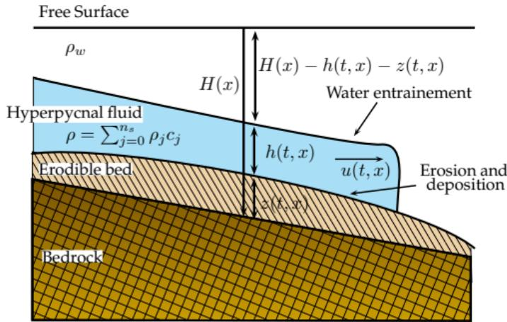
$$\left\{ \begin{array}{l} \partial_t h + \partial_x(hu) = \phi_\eta + \phi_b, \\ \partial_t(hu) + \partial_x \left( hu^2 + g(R_0 + R_c) \frac{h^2}{2} \right) = \\ \qquad g(R_0 + R_c) h \partial_x(H - z) + u \phi_\eta + \frac{u}{2} \phi_b + \tau, \\ \partial_t(hc_j) + \partial_x(hu c_j) = \phi_b^j, \text{ for } j = 1, \dots, n_s \\ \partial_t z + \xi \partial_x q_b = -\xi \phi_b. \end{array} \right.$$
